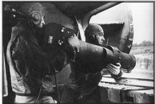
ABOVE: VD-1 photographers demonstrate an “oblique” camera rig with a 40-inch lens shooting through the side machine-gun port of a PB4Y-1. US Navy photo
